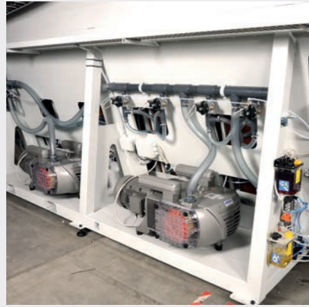
Vacuum pumps integrated in the machine frame
