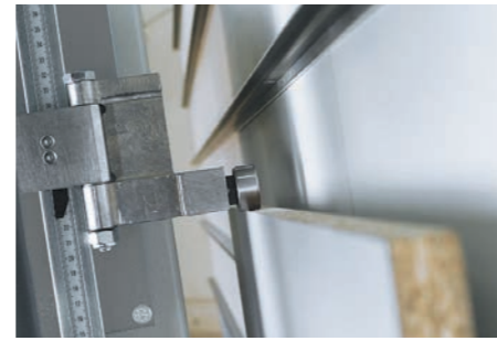
Repeat cutting device of horizontal strips
