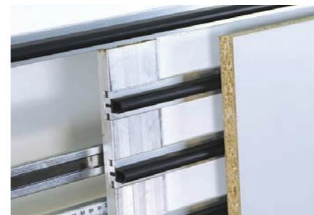
Sliding support for narrow pieces
