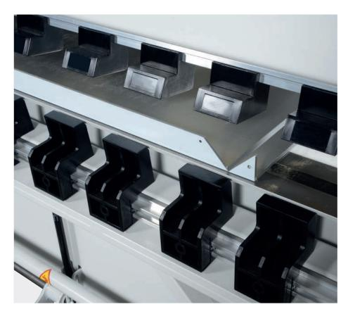
Bends the returning folds of the composite panels with aluminum skins (ACM, ACP, MCM) previously fabricated on a Panel Router, Alu Bender or a vertical panel saw.
