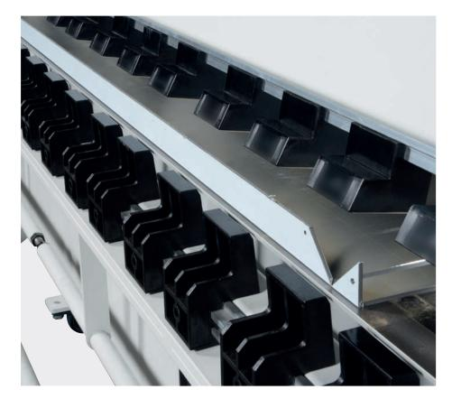
The locking and folding feet are completely adjustable and are made of plastic that will not mark or scratch the surface of the composite panel during the bending process, even when folding of all four sides.
