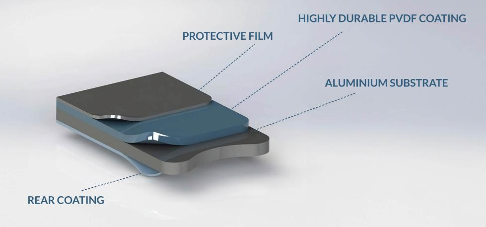
Futural is solid aluminium cladding panel that is **A1 non-combustible to BS EN 13501-1** and suitable for any type of buildings at any height. Made from 5000 marine grade aluminium with PVDF coatings, it is highly durable and impact resistant, yet available in unlimited colour range with superior surface and weather resistance.
