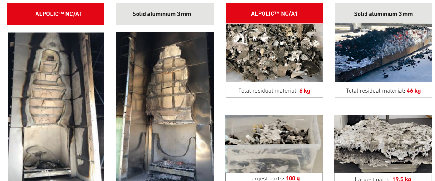
Result after a large-scale fire test (BS8414-2)
