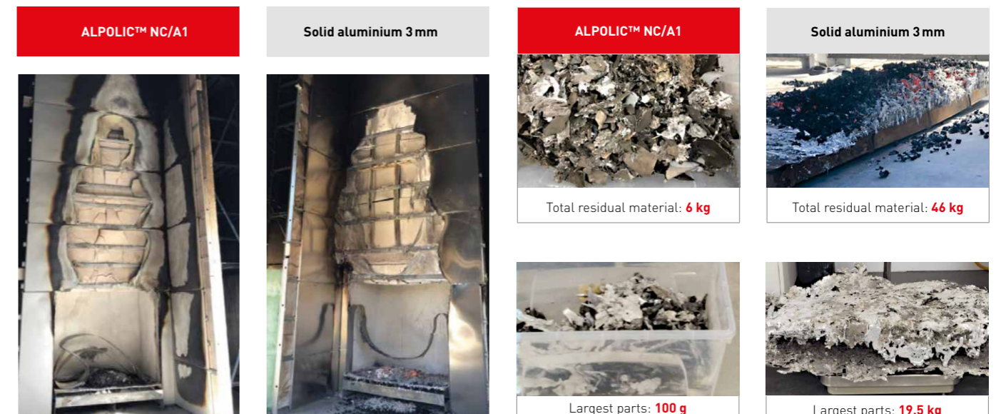
Result after a large-scale fire test (BS8414-2)
